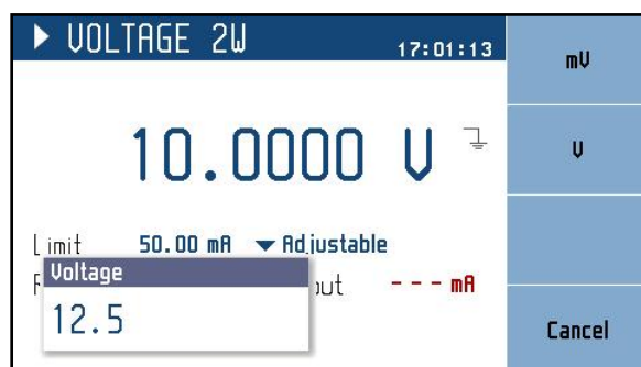
Figure 22 Numeric value entry
