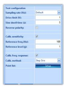
• Configurable profile for Swept Sine FRF measurement
