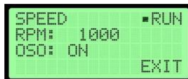
Figure 53 Calibrator in the RUN Mode with OSO ® Output Enabled
