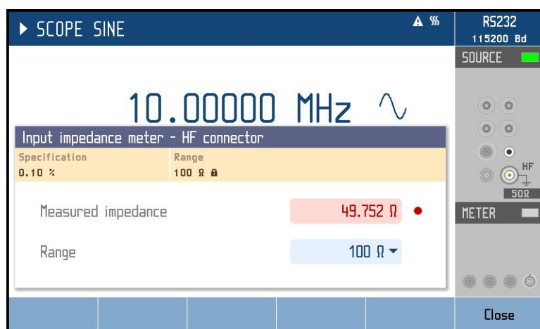
Figure 38 SCO option input impedance measurement
